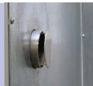
Exhaust air opening in the rear wall to vent the exhaust gases generated during drying
