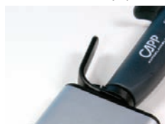
Lever for effortless tip ejection
